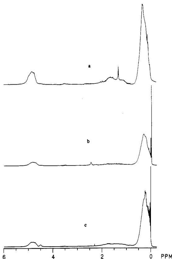
Figure 7. Liquid-state ^1\text{H} NMR spectra of (a) 8K MHPS polymer, (b) NCP100, and (c) NCP200.
